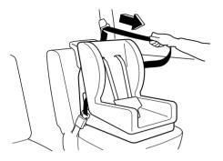
5. Push the child-restraint system firmly into the vehicle seat. Be sure the belt retracts as snugly as possible. A clicking noise from the retractor will be heard during retraction if the system is in the automatic locking mode. If the belt does not lock the seat down tight, repeat this step.
